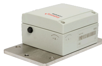
Wireless tiltmeter mounted on a versatile horizontal surface mounting plate (LS-ACC-IN15-HP). The plate has three clearance holes for M8 anchor rods and a M8 threaded hole allowing a combined use with surveying.
