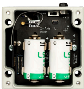
An inner view of a LoadSensing wireless tiltmeter.
