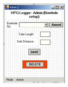
Having defined the number of profiles for the current site on the previous screen, this is where the profile details are entered: Tube Length and Start Distance. Other parameters for a reading run, such as the number of reference readings to be taken and the interval (distance) between readings are set up for each individual run when in "User" mode.
