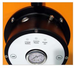
Close Up view of charger socket (see section 11) and Schrader valve for nitrogen/air pressure recharging (see section 12)
