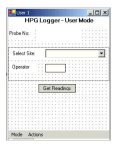
When this screen is first entered, the Field PC will interrogate the reel and retrieve the probe calibration data from it, to apply to the readings. If there is any problem with this step, the "Get Readings" button will not be available. If the problem is with the data returned from the reel, an appropriate error message will be displayed.
