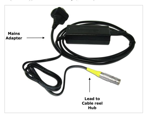
To charge from the mains, plug the Lemo plug (sleeved plug pictured above and below) into the socket in the centre of the reel hub, ensure the system is turned off and then connect the mains adapter to the mains power outlet. The charge indicator on the charger will light red to indicate charging is taking place and then become green once the charge is complete.
