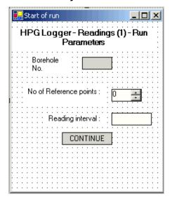
This screen is used to set up the number of reference (zero correction) points and the interval (distance) between readings. It will default to the first profile in the list, but this can be changed by selecting the appropriate one from the drop-down list. If this is done, when the screen is completed and the user is taken through to User Screen 2, the selected profile will be remembered.
