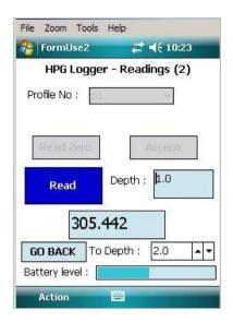
The User Screen shows a Battery Level bar. Once a reading has been taken (in other words, data have been sent back from the reel), the user screen will show this bar indicating the reel battery level. The bars start and end voltages are 13v (right hand end) and 11v (left hand end). It does not change colour at all – the indication of the state of the battery is the position of the bar.
