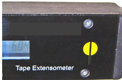
During this operation, the Tape Extensometer should be physically moved either side of the median position to ensure that any hysteresis within the instrument is eliminated. The correct tension is obtained when there are no visible yellow on either side of the black cursor line, and when any slight displacement to the extensometer reads as a positive displacement of the cursor line.
